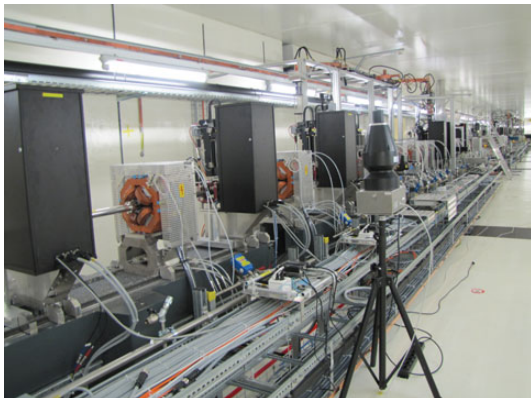
Figure 1. Experimental set-up exemplarily described by the diagnostic section of the accelerator with measurement position ‘Diag’ and the LB6419 neutron detector.
