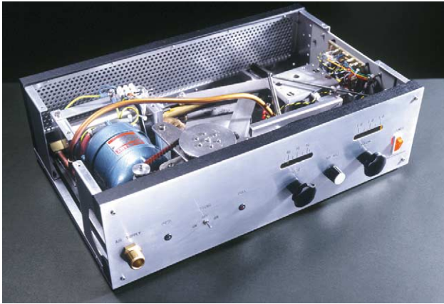
Fig. 5. Purpose-built pump to regulate heart rate, stroke volume and arrhythmia induction.
