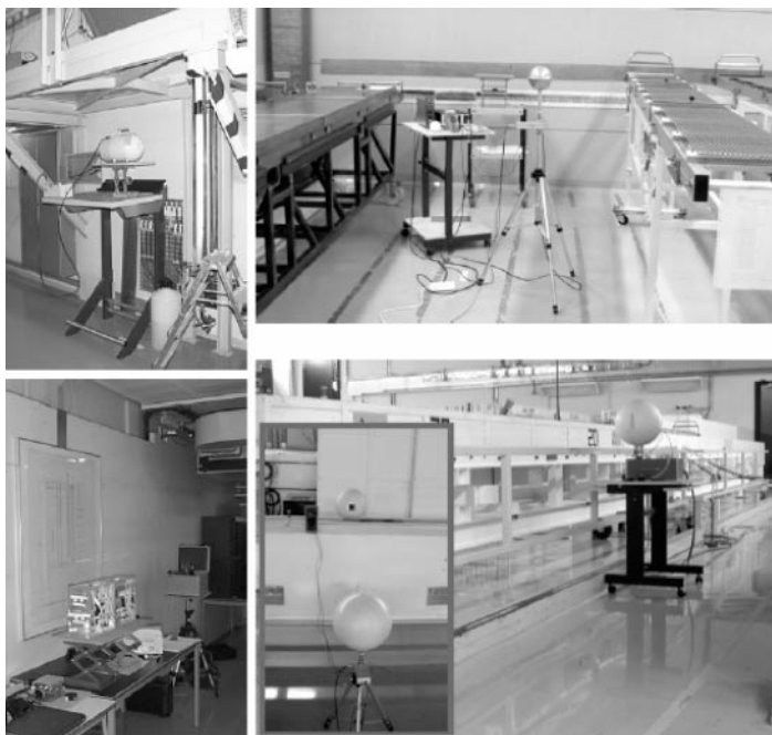
Figure 2. Workplaces investigated during campaign C2 in Mol, Belgium: (a) The field SCK•CEN VENUS F was next to the concrete shielding wall of the reactor, at the height of the core; (b) SCK•CEN VENUS C was located behind an additional polyethylene shield protecting the workers in the control room during a reactor run; (c) Belgonucléaire 1 was located in the proximity of a rack holding bare MOX fuel rods; (d) Belgonucléaire 2A and 2B were on the two sides of a rack (one shielded and one unshielded) where fuel boxes are manipulated before they enter the storage room.
