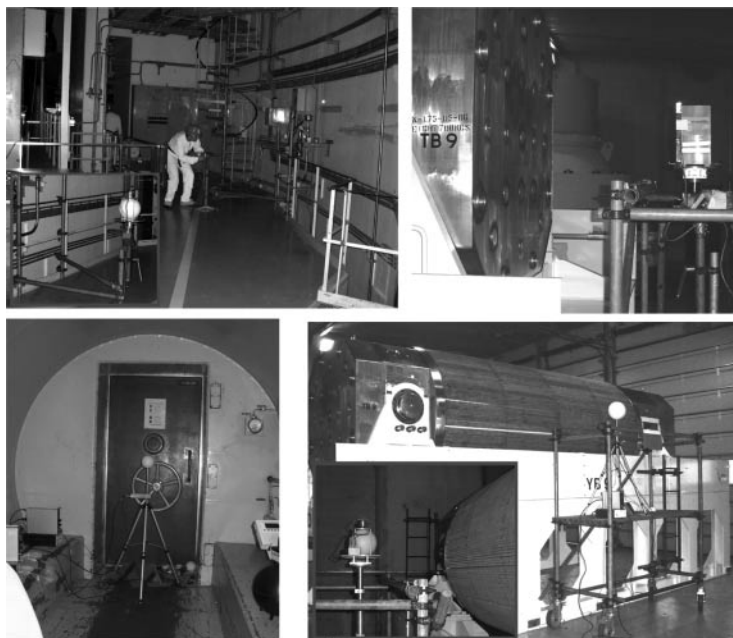
Figure 3. Workplaces investigated during campaign C3 at Ringhals, Sweden: (a) The field PWR Ringhals A was located inside containment a few meters above the core; (b) PWR Ringhals L was located close to an entrance lock door; (c) Cask TN N was located at the centre of the end plate of the cask; (d) Cask TN D was located at the centre of long side of the cask.
