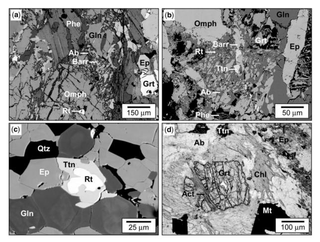
**Fig. 3.** Typical retrograde overprints. (a, b) Backscattered SEM images of albite and barroisite symplectite overgrowths on omphacite in massive eclogites GR 29 and GR 21. (c) Backscattered SEM image of titanite overgrowth on rutile in the rock matrix of massive blueschist GR 02. (d) Typical retrograde assemblage of massive greenschist GR 23 composed of albite, chlorite, actinolite and magnetite replacing garnet (see the section 'Petrography').
