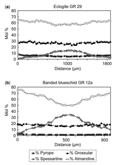
Fig. 7. Chemical zoning of garnet from the massive eclogite GR 29 and the banded blueschist GR 12a. The prograde chemical zoning, defined by the rimward decrease of the spessartine and increase of almandine components, is generally more pronounced in the banded rocks than in the massive rocks.
