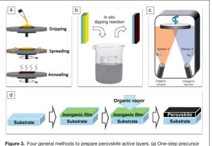
**Figure 3.** Four general methods to prepare perovskite active layers. (a) One-step precurso deposition; (b) sequential deposition method; (c) dual-source vapor deposition; and (d) vapor-assisted solution process. Reprinted with permission from Reference 15. © 2014 Royal Society of Chemistry.
