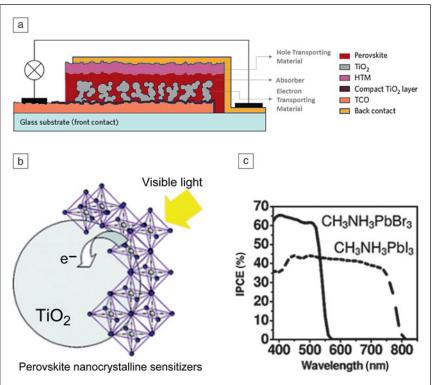
**Figure 1.** (a) A schematic illustration of a perovskite-sensitized solar cell. (b)  $TiO_2$  undergoing photoexcitation and electron transfer. The filled circles represent iodide, and the empty circles represent lead. (c) The incident photon-to-electron conversion efficiency (IPCE) spectra for perovskite-sensitized solar cells. Reprinted with permission from Reference 4. © 2012 AAAS. Note: HTM, hole transport material; MAI, methylammonium iodide; TCO, transparent conducting oxide.
