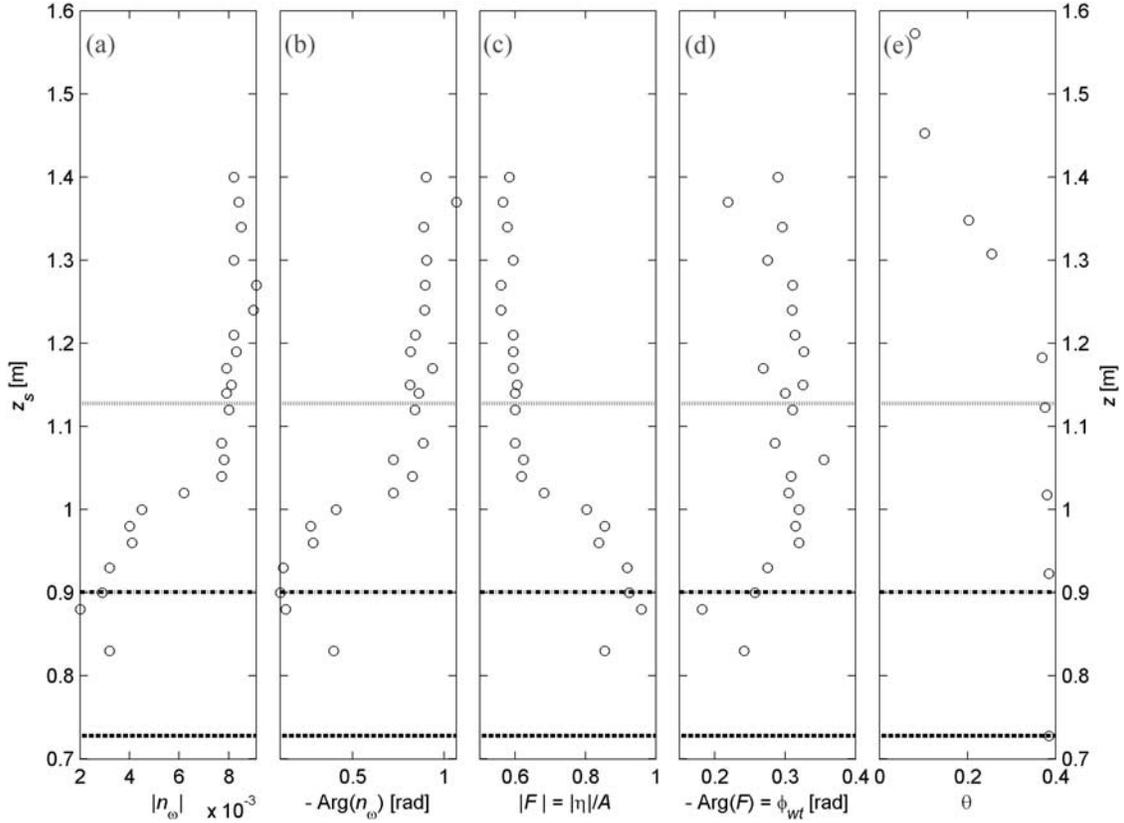
**Figure 3.** Influence of a truncated capillary fringe on (a)  $|n_\omega|$ , (b)  $-\text{Arg}\{n_\omega\}$ , (c)  $|F|$ , and (d)  $-\text{Arg}\{F\}$ . Also shown is (e) the equilibrium first drying curve, where  $z = D + \psi$ . The horizontal curves in each plot represent the mean driving head level,  $D$  (solid curve), the maximum driving head elevation,  $D + A$  (dash-dotted curve), and the equivalent saturated height of the equilibrium total moisture,  $D + H_\psi$  (dashed curve).
