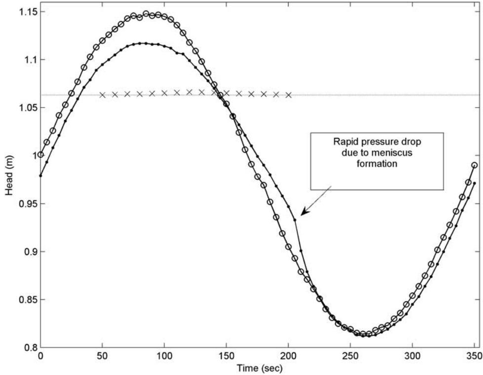
**Figure 4.** Observed time series from the sand column indicating the effect of meniscus formation at the sand surface. The different curves denote the driving head  $h_0$  (solid curve with open circles), the piezometric head  $h^*(z_0 = 0.4 \text{ m})$  (solid curve with closed circles), the free surface observed above the sand surface (crosses), and the sand surface elevation  $z_s = 1.063 \text{ m}$  (dotted line).
