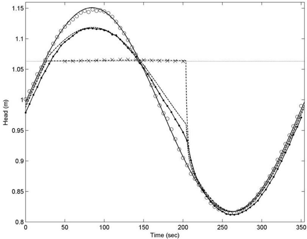
**Figure 7.** Comparison between the numerical Richards equation model results and experimental data. The curve and symbol types are defined for the driving head (open circles, observed; solid curve, fitted), the piezometric head  $h^*(z_0 = 0.51 \text{ m})$  (solid circles and curve, observed; dashed curve, simulated), the observed free surface (crosses), simulated  $h(h_{tot})$  (dash-dotted curve), and the sand surface (dotted line).
