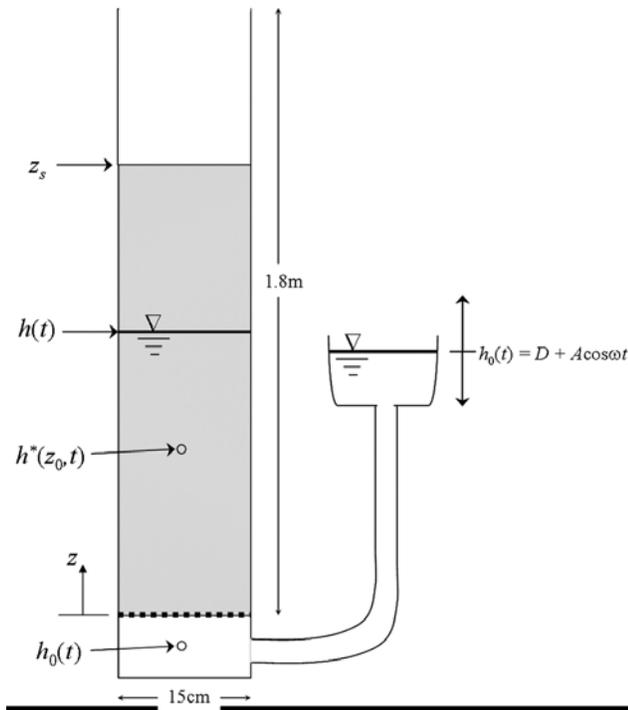
**Figure 1.** Schematic of the experimental sand column.
