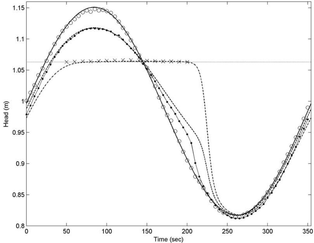
**Figure 5.** Comparison between the simple wetting and drying model results and experimental data. The curve and symbol types are defined for the driving head (open circles, observed; solid curve, fitted), the piezometric head  $h^*(z_0 = 0.4$  m) (closed circles with solid curve, observed; dashed curve, simulated), the observed free surface (crosses), simulated  $h(h_{tot})$  (dash-dotted curve), and the sand surface (dotted line).
