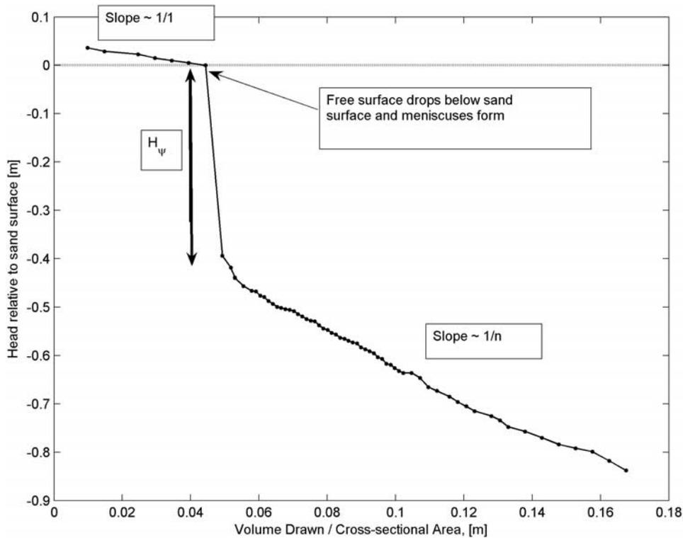
**Figure 2.** Pore pressure head variation with the equivalent depth of water extracted from the sand column. Note the disproportionately large pressure drop after the removal of only a minute volume water as meniscuses form at the sand surface.
