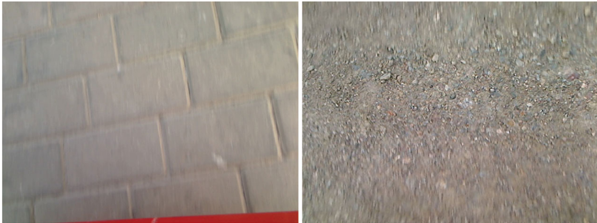
Fig. 5. (Colour online) Images taken by the camera pointing at the ground (velocities > 1 m/s): (a) Blur effect (flat terrain); (b) vibrations effect (bumpy terrain).
