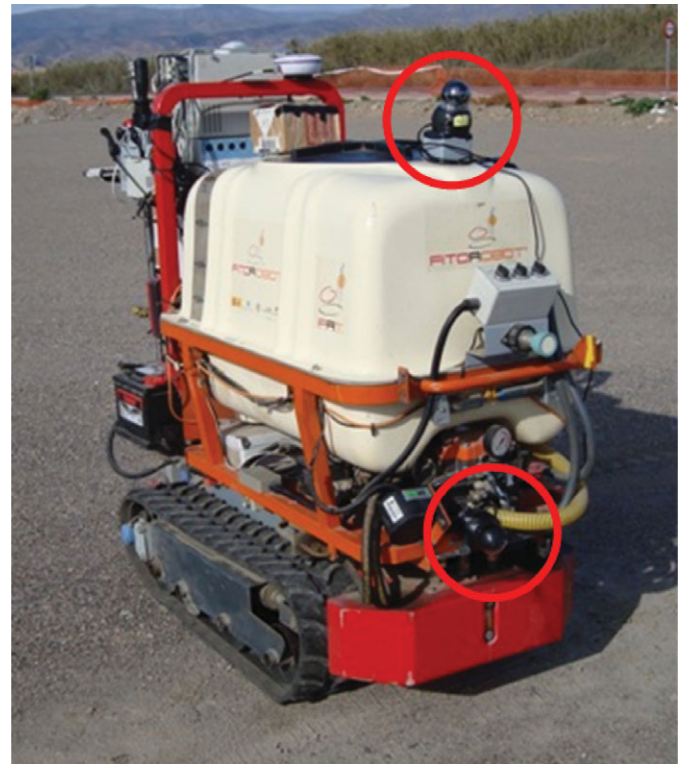
Fig. 4. (Colour online) Tracked mobile robot Fitorobot at the experiment site. Observe the position of the two cameras on the robot.
