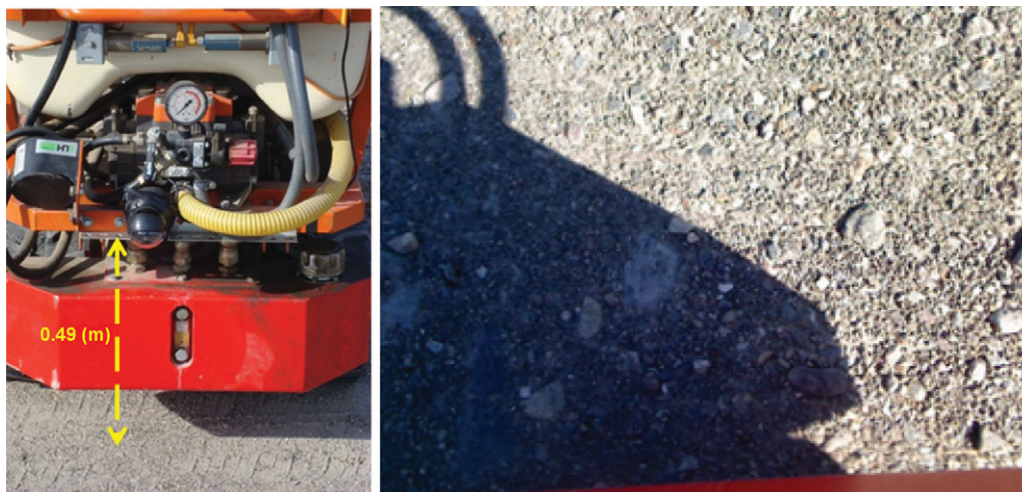
Fig. 6. (Colour online) Position and image acquired by groundcam with shadows. (a) Height of the groundcam. (b) Shadows in the groundcam.
