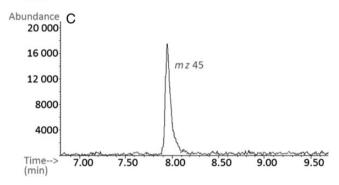
**Figure 1.** (A) Total ion current (TIC) chromatogram of 25.0 nmol propane with 25 nmol deuterated propane, and the gray peak corresponds to propane. Extracted ion chromatograms of propane (m/z=44) (B) and deuterated propane (m/z=45) (C) obtained from the TIC chromatogram.
