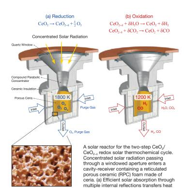
while product gases H2 and/or CO exit the cavity through an axial outlet port. Inset: Ceria RPC. Courtesy of ETH Zürich.
