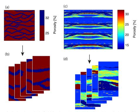
Figure 3. Training images for the channels case (a), the fluvial deposits case (c) and multiple-point statistics realizations thereof (b and d). Note that the full ensemble of TI realizations contains 1000 realizations for both cases.
