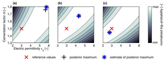
Figure 12. Maps of the posterior log-probability for all possible combinations of the petrophysical parameters m and  $\varepsilon_s$  for the fluvial deposits case. The DCT coefficients are fixed at their maximum a posteriori density (MAP) values. Indicated are the parameter values of the reference (red crosses), the values for which the log-probability is maximized (black crosses) and the estimate found by DREAM<sub>(ZS)</sub> (blue asterisks). Enumerations correspond to those of Fig. 11.
