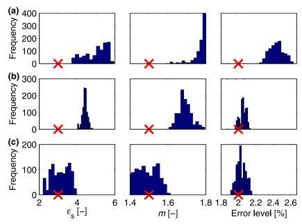
Figure 11. Posterior distributions of the petrophysical parameters  $\varepsilon_s$  and m, and of the relative data error level for the fluvial deposits case: (a) no TI-based parametrization, no summary metric prior, (b) TI-based parametrization, no summary metric prior and (c) TI-based parametrization, summary metric prior using roughness and percentile metrics. Red crosses depict the reference values.
