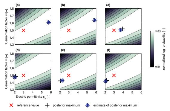
Figure 7. Maps of the posterior log-probability for all possible combinations of the petrophysical parameters m and  $\varepsilon_s$  for the channels case. The DCT coefficients are fixed at their maximum a posteriori density (MAP) values. Indicated are the parameter values of the reference (red crosses), the values for which the log-probability is maximized (black crosses) and the estimate found by DREAM<sub>(ZS)</sub> (blue asterisks). Enumerations correspond to those of Fig. 6.
