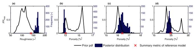
Figure 13. Prior probability density functions derived from the distribution of summary metrics in the ensemble of TI realizations (black lines, see Fig. 2 for explanation) and the posterior distributions of the summary metrics (blue bars) for the fluvial deposits case: (a) roughness metric, (b)–(d) 10, 50 and 90 per cent percentile metrics. Red crosses depict the summary metrics of the reference porosity field.
