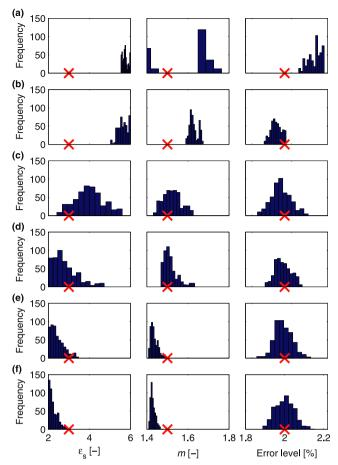
**Figure 6.** Posterior distributions of the petrophysical parameters  $\varepsilon_s$  and m, and of the relative data error level for the channels case: (a) no TI-based parametrization, no summary metric prior, (b) TI-based parametrization, no summary metric prior using (c) roughness metric, (d) variability metric, (e) percentile metrics, (f) both variability and percentile metrics. Red crosses depict the reference values
