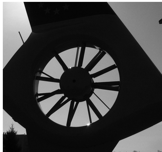
Fig. 5. Asymmetric and encapsulated Fan-in-Fin-Rotor Fenestron® heck rotor of EC 135.
