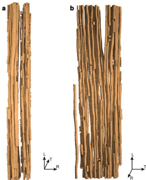
Figure 3 Vessel network of beech wood looking along T-direction (a) and R-direction (b). Sample height is 3 mm. Note that the displayed vessel discontinuities are mainly as a result of vessels moving in and out of the extracted volume.
