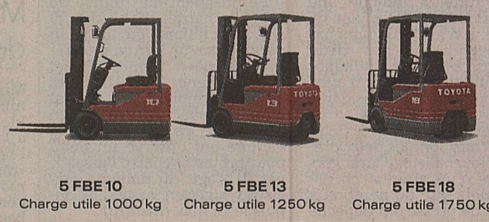
5 FBE 10 Charge utile 1000 kg | 5 FBE 13 Charge utile 1250 kg | 5 FBE 18 Charge utile 1750 kg
