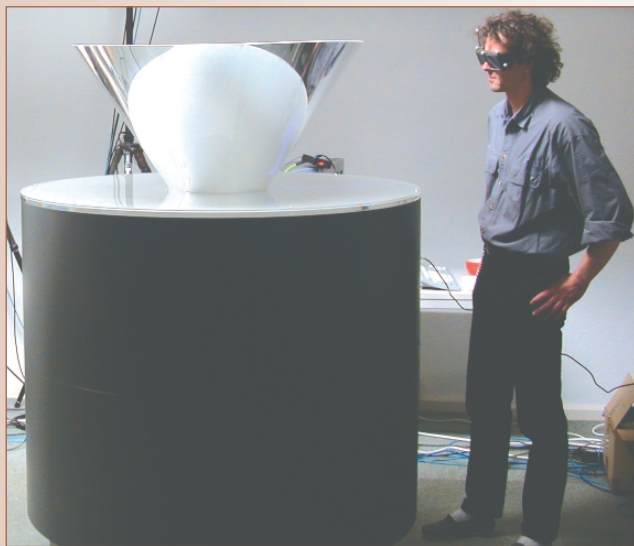
Figure A. Virtual Showcase. This example of a cone-shaped prototype supports two to three users, wireless user tracking, and a seamless surround view.
