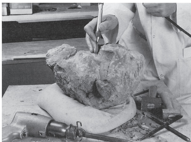
Fig. 1 A hand-held, pneumatic engraving pen used to remove rock matrix. In the foreground is a heavy duty pneumatic chisel.
