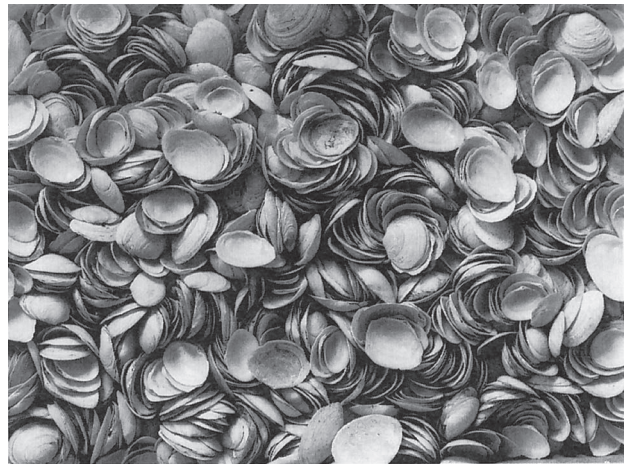
Fig. 2 Mainly vertically packed and tightly nested shells of Macoma balthica forming a beach deposit in a laboratory wave tank.
