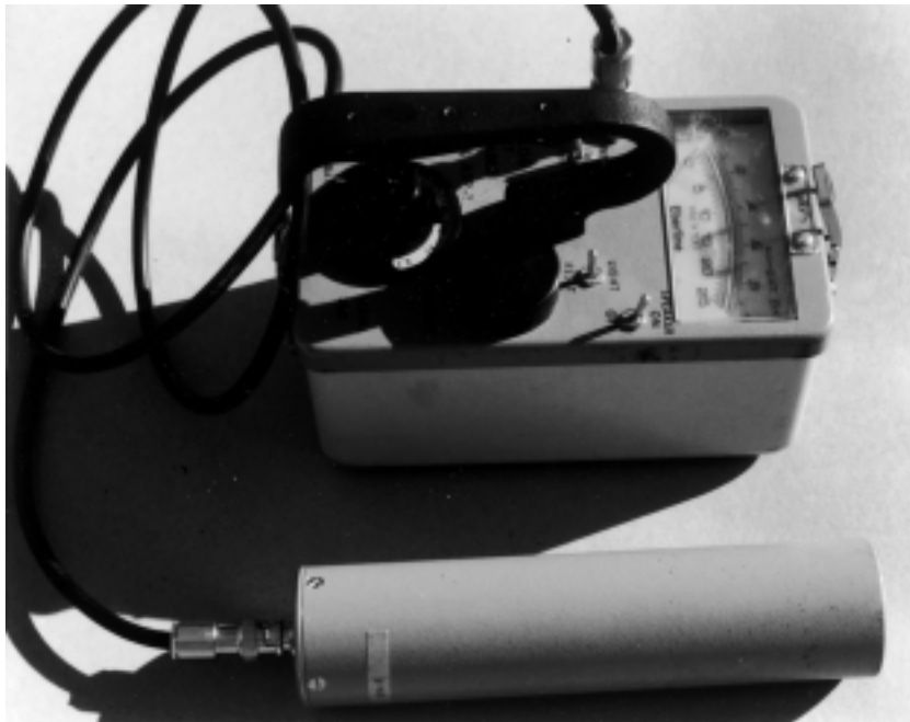
Fig. 1 - Eberline Analog Smart Portable Micro-Roentgen survey meter with a model SPA-8 sodium iodide detector.
