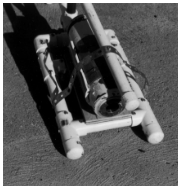
Fig. 3 - Underside of the lead shield and the 2.5 cm window for the sodium-iodine detector.
