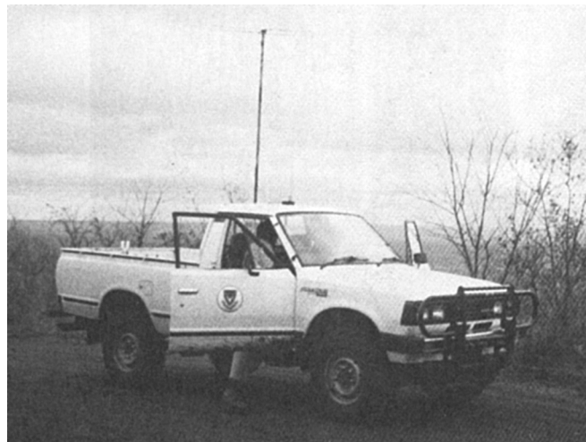
FIGURE 6. Mobile radio-tracking tower [15]
