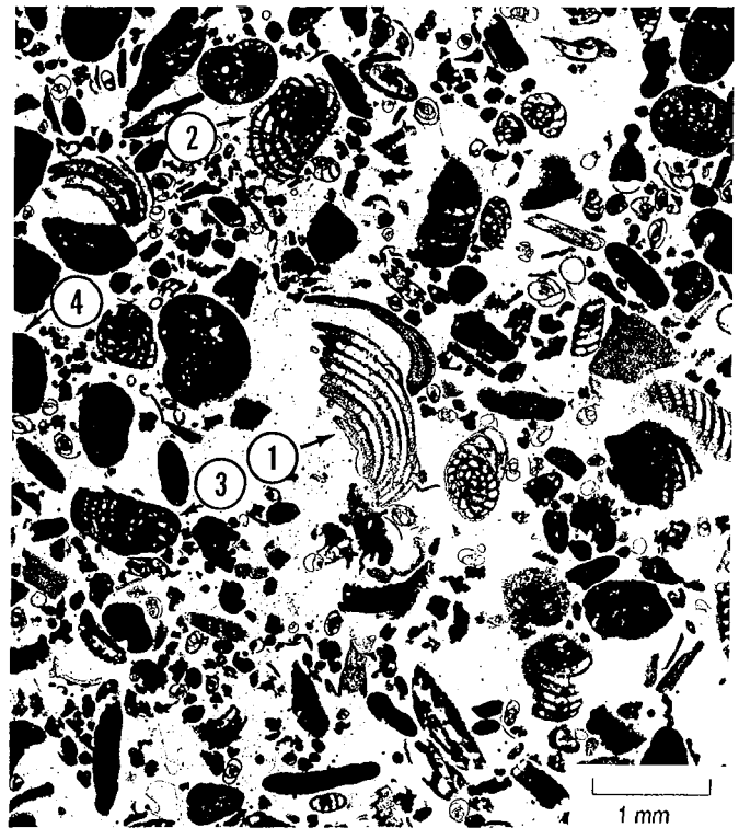
FIG. 4.—Sand-size fraction from the laminated miliolid-mud facies showing a marked increase in the alteration of peneroplid foraminifera with a decrease in grain size (note sequence indicated by arrows). Petrographic thin section, plane-polarized light.
