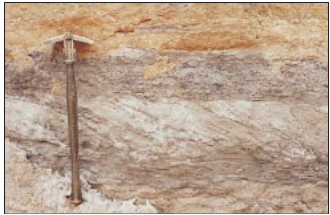
Figure 15. Photograph of the interbedded sand and mud. Light-colored laminae are sands; darker-colored laminae are clay drapes and silty clay laminae. Location along the east wall. Dip of cross-bedding is to the south.
