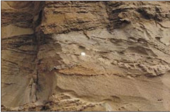
Figure 16. Photograph of the lower part of the cross-bedded sand. Clay draped laminae stand out in relief. Coin is a U.S. quarter, diameter approximately 1 in. Section located along the east wall.
