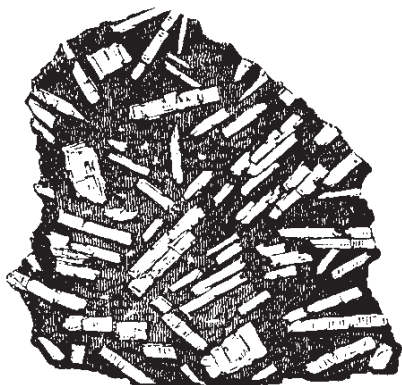
Fig. 634. White crystals of felspar in a dark base of hornblende and felspar.
