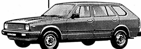
Datsun Cherry 1.3 GL break 1270 cm 3 , 44 kW (60 CV/DIN), 5 portes, 5 places, 5 vitesses
