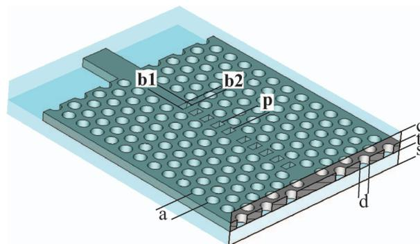
Fig. 1. In-plane photonic crystal microcavity structure buried in silicon dioxide (PhC period  $a=490$  nm, hole diameter  $d=350$  nm, core thickness  $t=238$  nm, bottom oxide thickness  $s\approx 2000$  nm, upper cladding thickness  $c\approx 700$  nm). The microcavity inside the photonic crystal waveguide is formed by two five-hole Bragg reflectors (hole dimensions  $b1=325$  nm and  $b2=180$  nm, period  $p=373$  nm).
