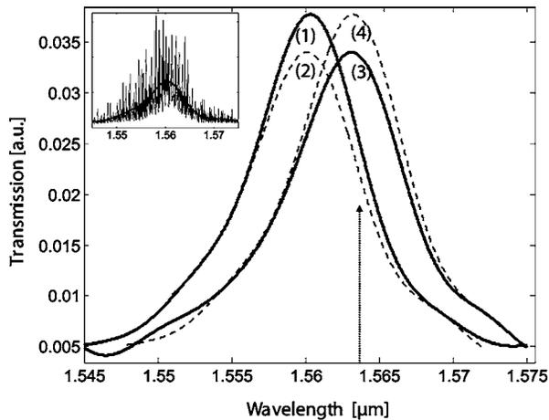
Fig. 2. Measured transmission spectra through the photonic crystal microcavity (1) without and (3) with the control laser illumination ( $\lambda = 532$  nm). Curves (2) and (4) approximately indicate the change induced by the plasma dispersion and thermo-optical effects, respectively. The arrow indicates the fixed wavelength for the temporal response measurements. The inset depicts the unfiltered transmission spectrum with the periodic Fabry-Perot interference oscillations.
