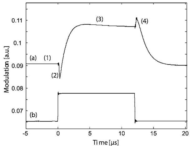
Fig. 3. (a) Measured temporal response of the transmission signal with its switching characteristics [positions (1) to (4)]. The slight decrease of the signal in position (3) is most likely due to secondary thermal effects induced in the bulk silicon. (b) Square modulation pulse applied to the control laser.
