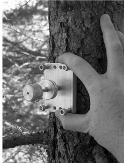
Figure 1. Increment puncher used for collecting minute samples of tension wood (Forster et al. 2000).
