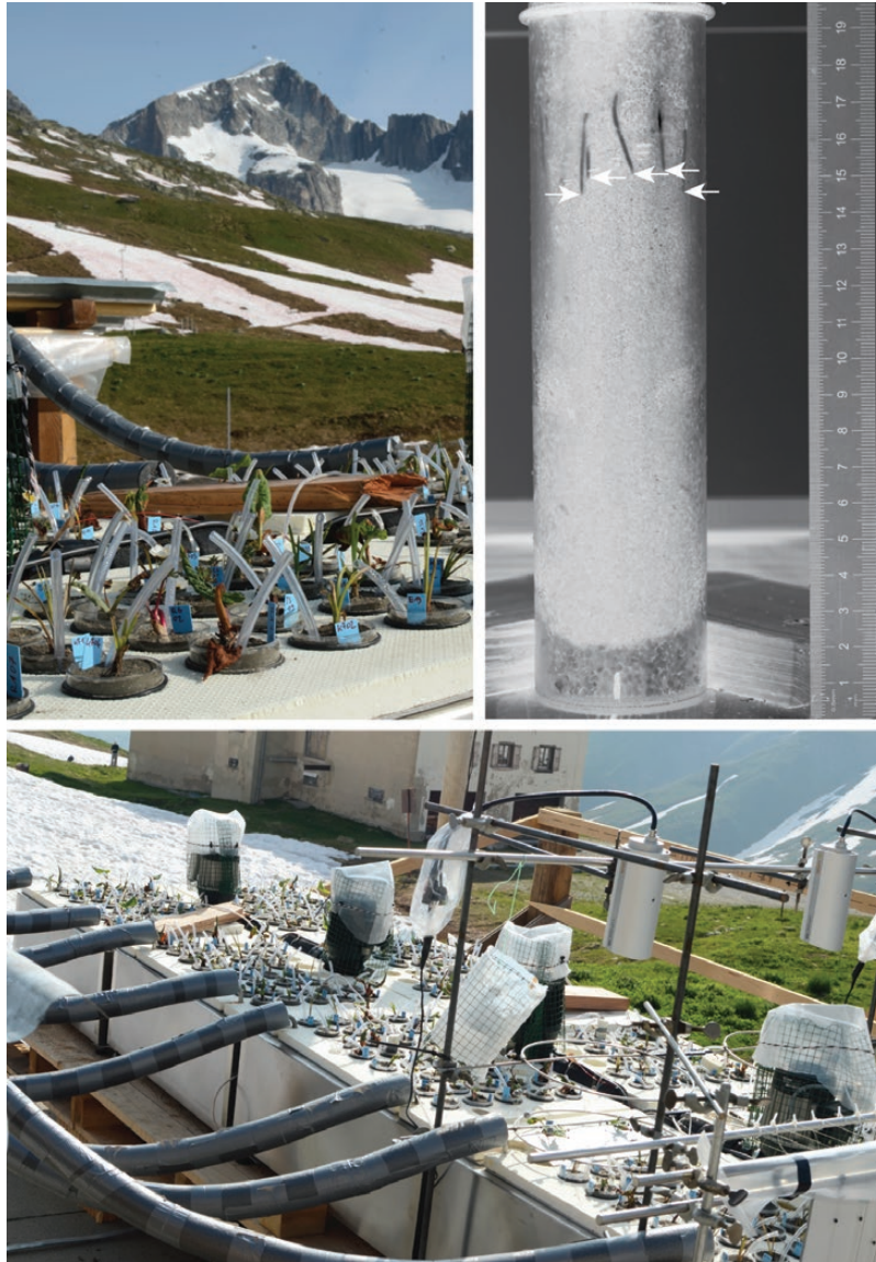
Figure 2. Thermostated water bath systems at the Furka Pass (2440 m a.s.l.) with transparent cylinders for root observation (measurements of RERs). The black to white converted image of a root cylinder taken in a photo box shows roots of Rumex alpinus growing along the wall. White arrows point at root tip positions.
