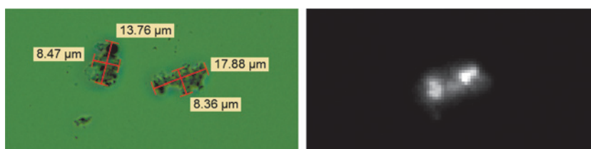
Figure 4: An example of a dig of size 5/1 \times 0.016 on a planar mirror. On the left under a microscope and on the right with our dome.
