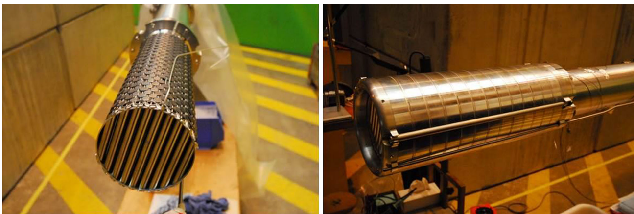
Fig. 5 Actually used SINQ target design MARK IV. Left Rods mounted in target holder. Right Target surrounded by Pb blanket
