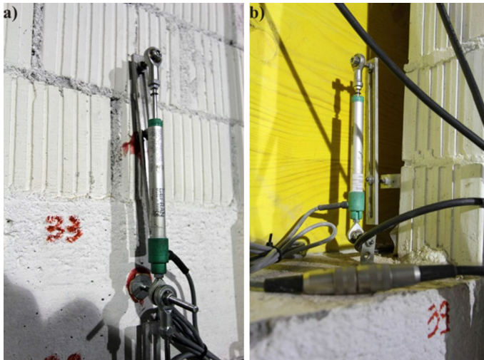
Fig. 36 Potentiometers measuring the relative rotation between slab and out-of-plane loaded wall: “Pot_33” (a) and “Pot_39” (b) measuring base rotation of the third-storey URM walls on the north face of the building
