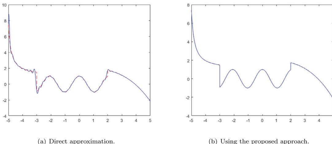
**Fig. 2.** Interpolation of the function  $f_1$  using 80 nodes and  $d = 8$  in the FH interpolant. In red the function and in blue the interpolant. (For interpretation of the references to color in this figure legend, the reader is referred to the web version of this article.)
