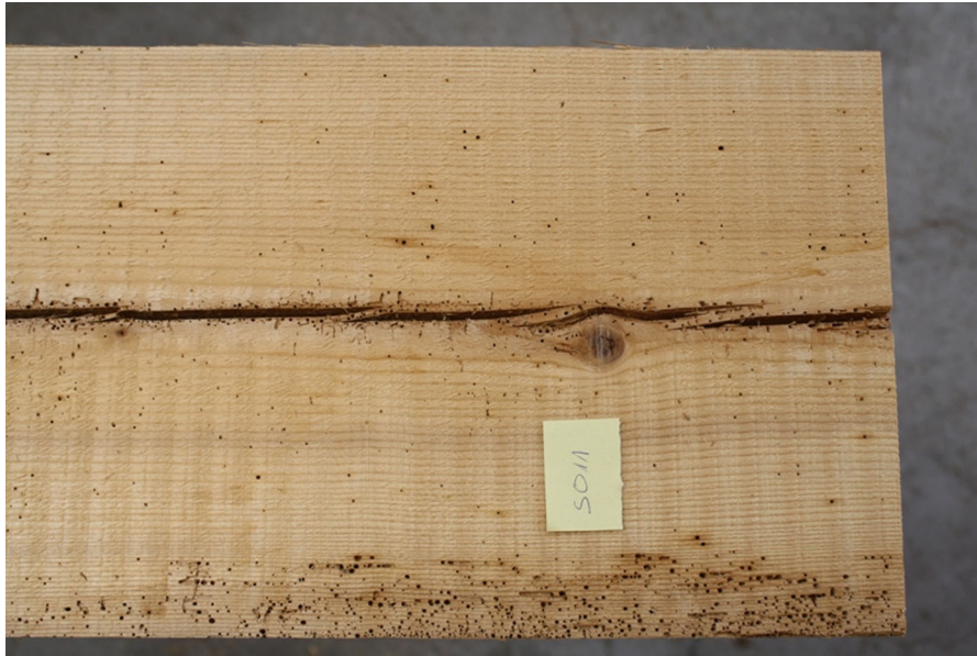
Fig. 2 Damage due to insect attack
