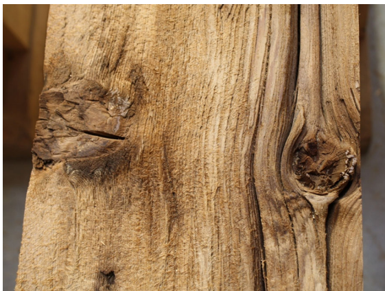
Fig. 1 Weathered surface of an aged board
