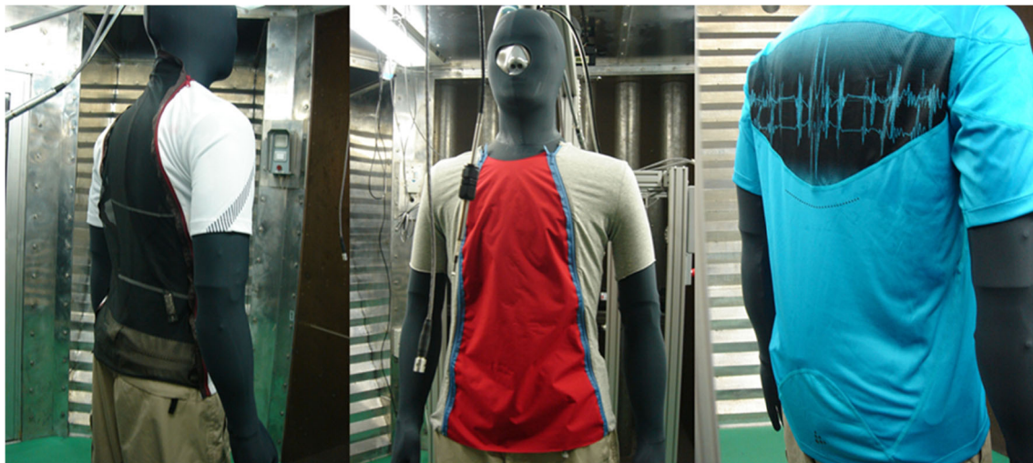
Fig. 1 The modular body mapping T-shirt ( left and middle ) and the commercial product ( right )
