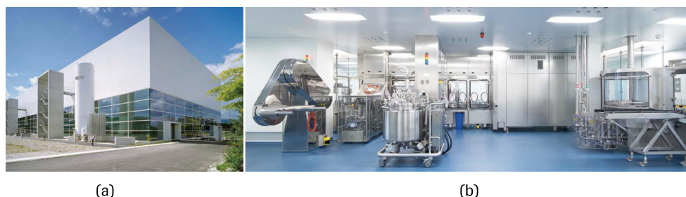
Fig. 2 Introducing parenterals production Kaiseraugst of F. Hoffmann-La Roche Ltd.: a facility exterior; b filling line of liquid vials using isolator technologies are found in first floor
