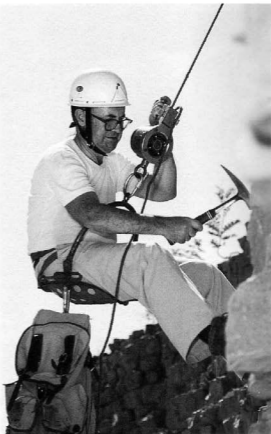
Fig. 4: Measuring a section on a light steel rope lined with nylon fabric. The steel seat is held steady by a clamp with wooden brake-shoes that may be fastened with a screw (lever held by the left hand). When descending, an automatic brake operating with the centrifugal force regulates the sinking speed to 1 m per second. This safety brake is in the circular casing beside the face. With this device it was possible to work with two free hands for measuring, taking samples and writing. When measuring long sections, a very high frequency (VHF) radio was used to dictate the text to be written into the fieldbook to S. Gysi (my wife).
