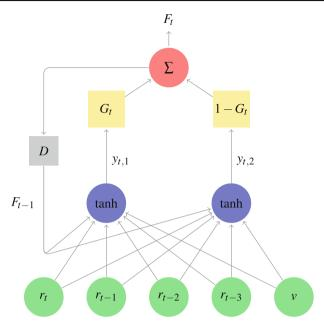
Fig. 1 RSRRL network structure where D is the delay operator and m = 4
