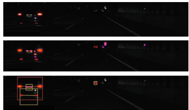
Fig. 2 Detection results: top row input frame, center row taillight detection, bottom row vehicle detection
