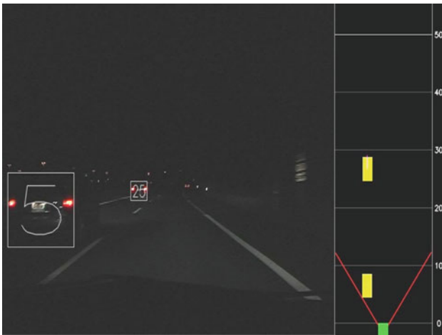
Fig. 1 Sample output of our real-time tracking system. On the left tracked vehicles are marked and their distance in meters to the camera is overlaid on them. On the right a radar-like view of the scene is drawn: the bottom rectangle represents the car on which the camera is mounted and other represent preceding vehicles. The short line segment on them indicates their relative velocity with respect to the camera
