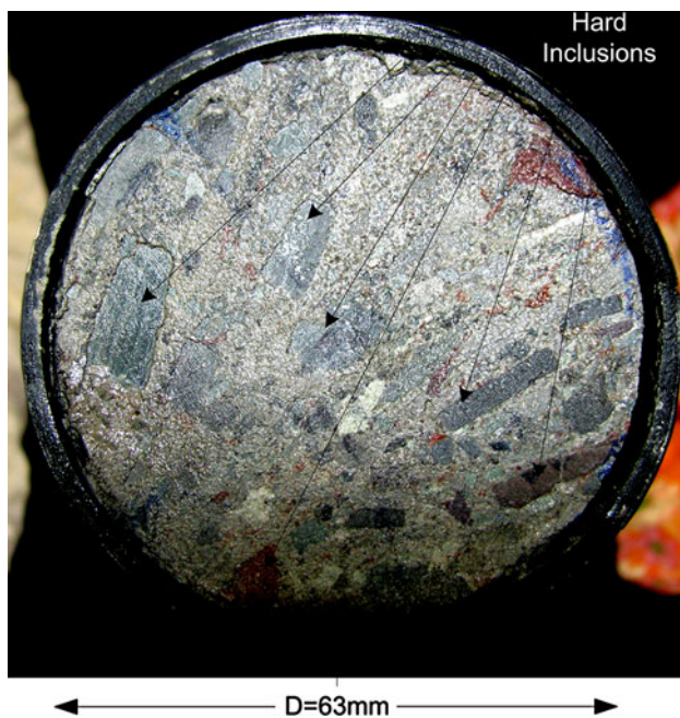
Fig. 4 Cross section of breccia core Z10
