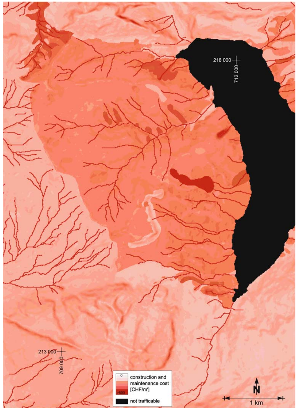
Fig. 7 Spatial variability in road life cycle costs for Scenario III, based on slope gradient and geotechnical soil properties. The lake "Wägital" (35 km 2 ) is at eastern boundary and watershed is at western boundary
