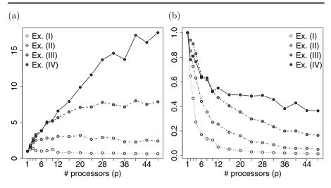
Fig. 8 Speed-up and efficiency for the new parallel algorithm based on lists and indexing trees: (a) speed-up, (b) efficiency
