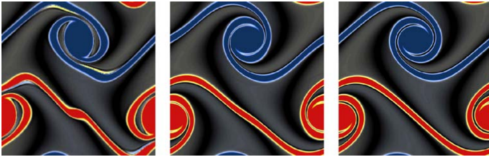
Fig. 4. Simulations of the thin double shear layer. Red denotes high positive vorticity, and blue denotes high negative vorticity. Left to right: simulation using 256 \times 256 , 512 \times 512 and 2048 \times 2048 particles. Note the development of a spurious vortex for the two lower resolutions
