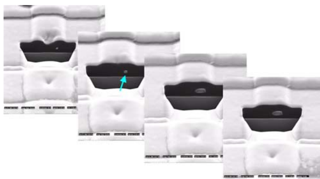
Fig. 7 Sliced FIB cross section through a poly fuse stringer, beginning at the center ( top left ), ending at the full size of the fuse's poly line ( right bottom )
