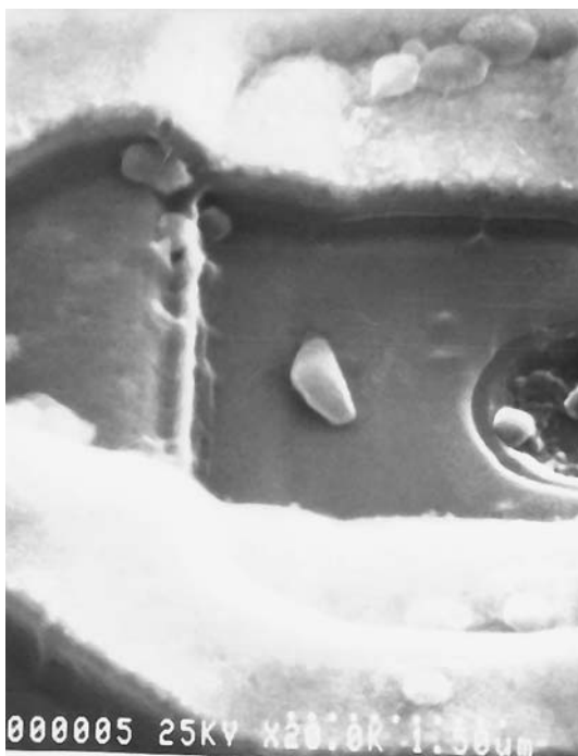
Fig. 4 Reoxidized Stringer, still performing a connection between the top and bottom polySi line
