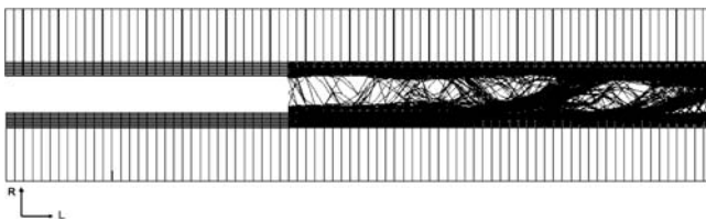
Fig. 12 Branching and bridging mechanism around the localized crack in whole fracture geometry
