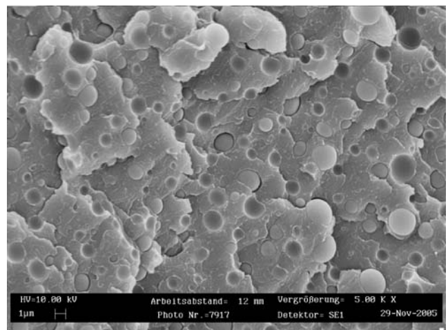
Fig. 6 Scanning electron micrograph of the PS/LLDPE 85:15 blend before elongation
