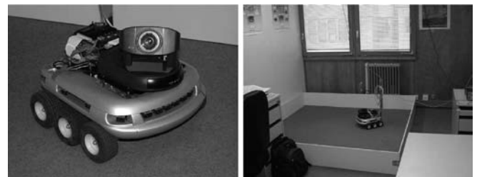
Fig. 14. Left: The Koala robot (produced by K-Team S.A.) equipped with a Sony EVI-D31 mobile camera and onboard PC-104 processor. The robot base is 30 cm w, 32 cm l, and 20 cm h; its total weight is 6 kg. Right: Evolutionary environment. The robot has visual access to the whole environment, but it can move only within the square arena. Lights were on day and night, and researchers and visitors were free to come to the office during the evolutionary process. The pole on the back of the robot prevents the aerial power supply cable from being trapped in the mobile camera. The other cable visible in this picture is used only after the evolutionary process to download data from the onboard computer to a desktop computer for analysis
