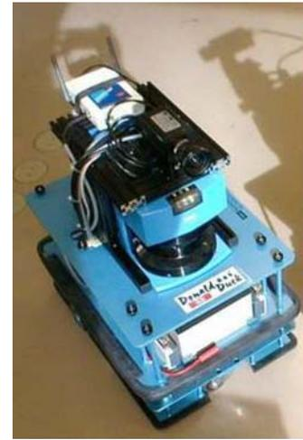
**Fig. 6** The autonomous robot Donald Duck. Its controller consists of a VME standard backplane with a Motorola PowerPC 604 micro-processor clocked at 300 Mhz. Among its peripheral devices, the most important are the wheel encoders, a 360° laser range finder and a grey-level CCD camera (not used here)
