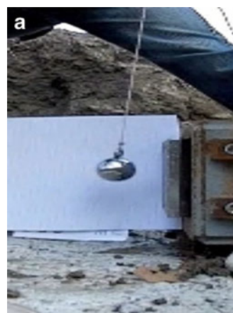
Fig. 4 a Setup for calibration tests of the pressure plates. b Force oscillation measured during one hard contact between the steel ball and the small pressure plate
