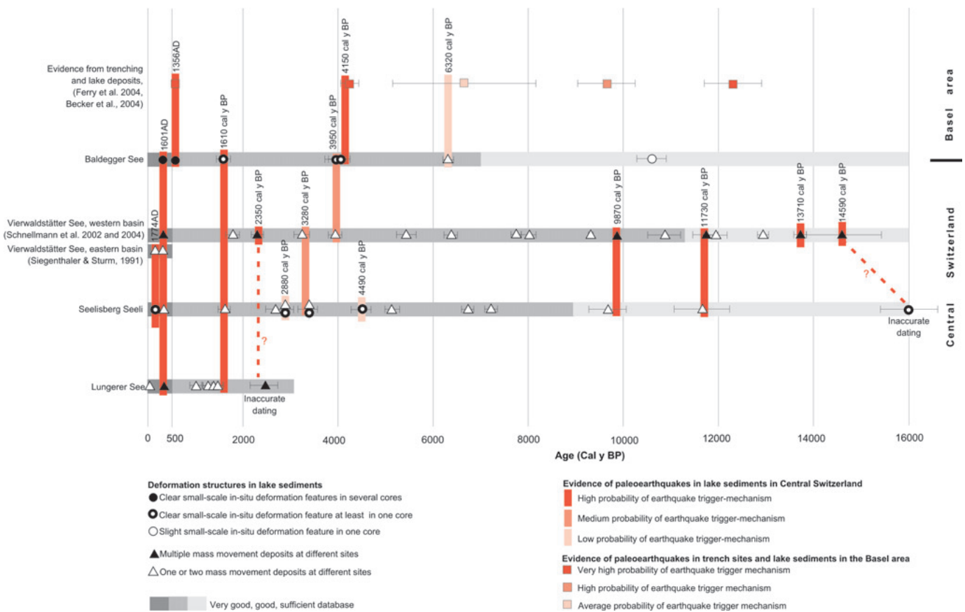
Fig. 16. Correlation of deformation structures in Vierwaldstätter See (after Schnellmann et al. 2006), Lungerer See, Baldegger See, Seelisberg Seeli and determination of historic and prehistoric earthquakes in Central Switzerland. Paleoseismic events with a high probability of a seismic trigger mechanism show clear evidence of earthquake-induced deformation at least within one lake or deformation structures within three or more lakes. Events with medium probability show a medium evidence of earthquake-induced deformation in one lake and further deformation in another lake. Events with low probability are visible only within one lake and show a medium evidence of earthquake-induced deformation. Deformation structures in Baldegger See partly correlate with paleoseismic events in the Basel area proposed by Ferry et al. 2004 and Becker et al. 2002.
