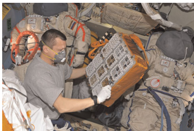
Fig. 2. Dmitry Kondratyev with Expose-R inside the ISS when the 22 month period of external exposure was over. The four brown-coloured windows are easily discernable. Credit: Roscosmos.
