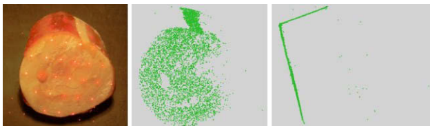
Figure 4: Result of scanning a wet bone with some flesh on it. Conditions as in figure 3.
