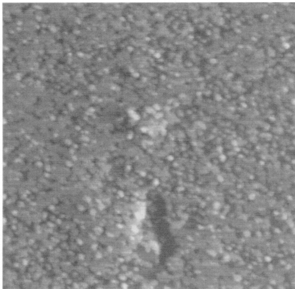
Fig. 13. In situ STM picture exemplifying the OPD copper layer-by-layer growth on a C_{10} thiolate-covered Au(111) electrode at 300 K. Electrode potential: -90 mV vs. Cu/Cu^{2+} . Electrolyte: 50 mM H_2SO_4 + 1 mM CuSO_4 . Tunneling parameters: I = 0.4 nA, V = 110 mV. Image size: 220 nm \times 220 nm.
