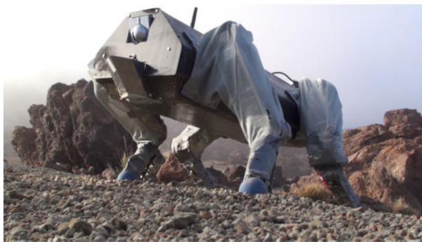
Figure 2 The quadruped robot ALoF. The robot is built with a classically stiff actuation in which joints, gearboxes, and motors are rigidly connected.
